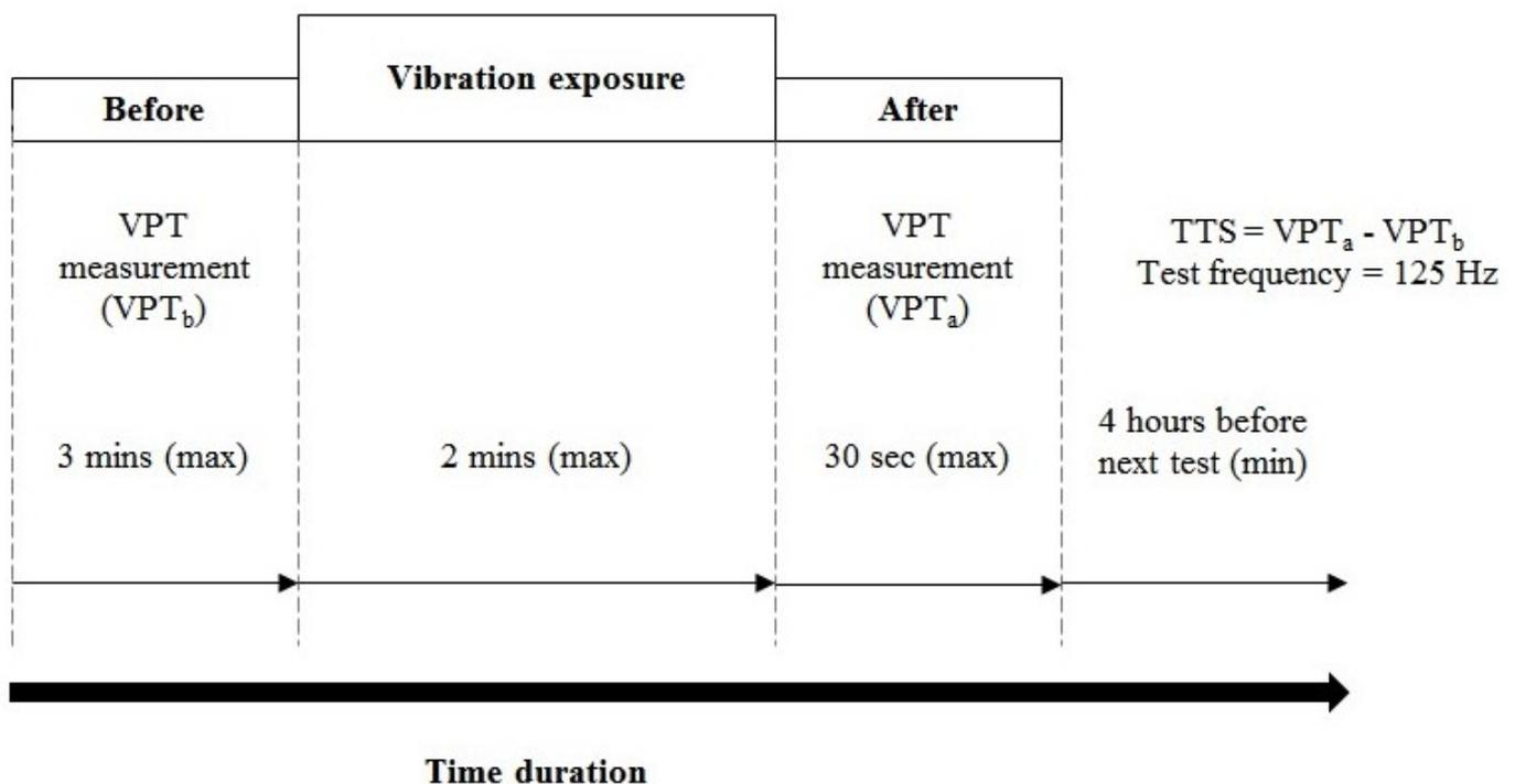
**Figure 1.** Experimental procedure for VPT measurement before and after tool vibration exposure.
