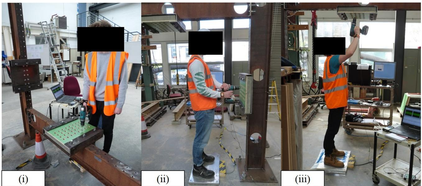
**Figure 2.** Test postures (i) vertical downwards similar to ISO 28527-5 posture, (ii) horizontal and (iii) vertical overhead.
