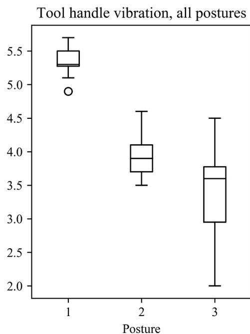
**Figure 3.** Tool handle vibration magnitude (ms<sup>-2</sup>) for all postures.
